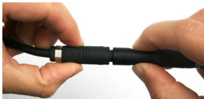
Fig. 1: Connection of Radox connectors showing ~2 mm gap
